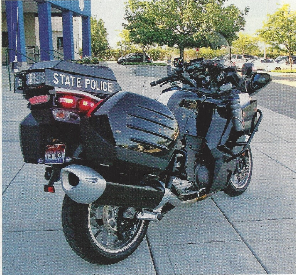
The Concours 14 uses a shaft drive and 4-link suspension to reduce squat and lift.
